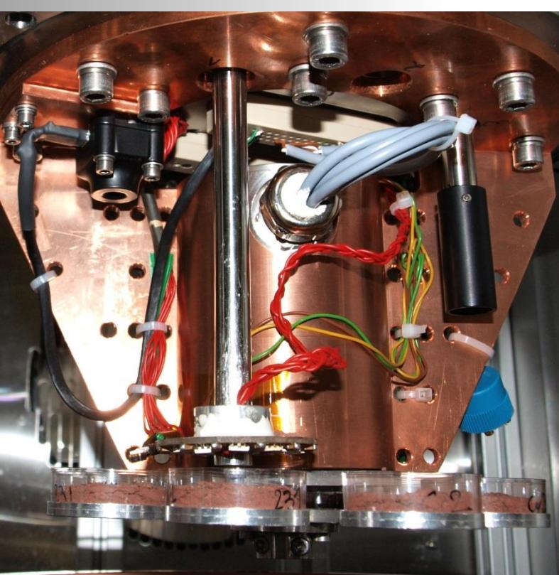
To analyze and document the processes, images are captured at regular intervals by a camera mounted in the simulation chamber. For the experiment, the researchers opted for a special industrial camera from IDS that combines two worlds: The USB 2 uEye XS.
