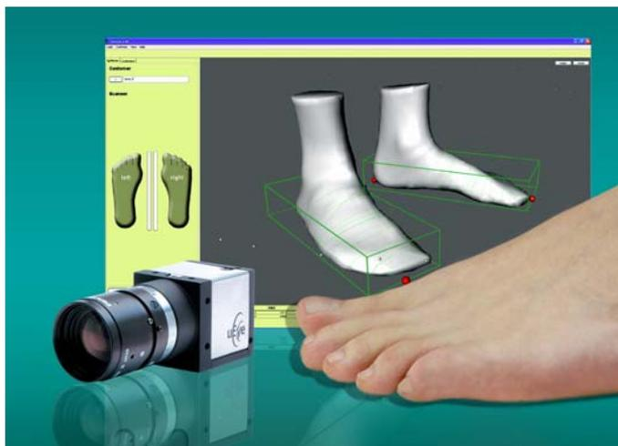
Approximately 150 different steps are required to craft a custom made shoe. A separate last must be formed for each shoe, for which the shoemaker takes measurements in 35 places. This elaborate procedure can now be handled by a foot scanner that not only speeds up the manufacturing process, but also makes it less expensive.
